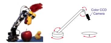
Fig. 5. A robot with four degrees of freedom used to capture images of objects. A small CCD camera is mounted in the right eyeball. A turntable provides a fifth degree of freedom for viewing objects from various perspectives. The turntable was only used for collecting images for the infant-directed speech experiments described in Section IX.
