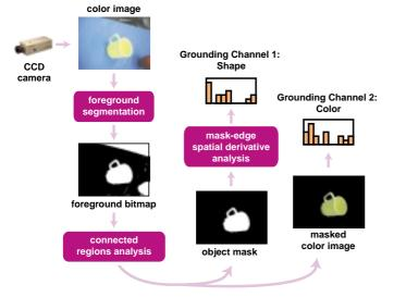
Fig. 4. Extraction of object shape and color channels from a  $\operatorname{CCD}$  camera.
