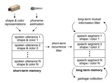
Fig. 3. The CELL model. A layered memory architecture combined with recurrence and mutual information filters (see text) are used to acquire an audio-visual lexicon from unlabelled input.
