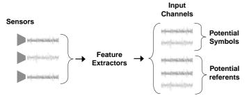
Fig. 2. Framework for learning from untranscribed sensory data. Feature detectors extract channels of input from sensors. The input channels are divided into two sets. The first carries symbolic information such as words and signed gestures. The second set carries representations of referents which may be associated with symbols. For example, visual channels may represent the shape or color of objects which are associated with shape and color symbolic terms.
